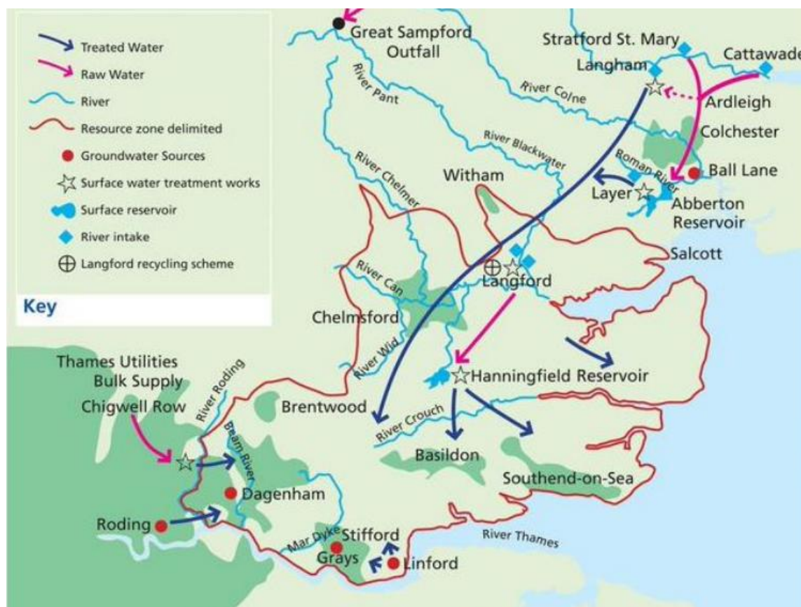
Figure 4 - Principal Features of the Essex WRZ (Source: Essex & Suffolk Water 4 )
